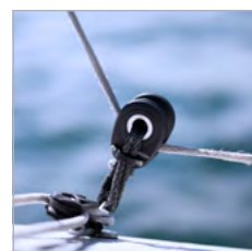
Cheek plates rotate to open block
